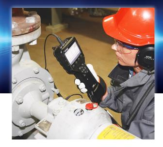
Leonova Diamond<sup>®</sup> incorporates highly advanced and innovative order tracking functionality. The powerful HD Order Tracking, applicable in an RPM range from just a few to thousands of revolutions per minute, enables more precise measurements and
