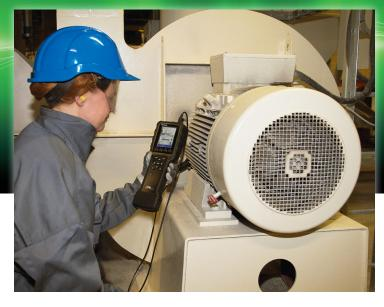
even where signals are weak and low in energy content. The 0 to 20 KHz frequency range covers most needs in practical vibration measurement.
